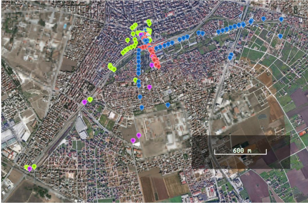
Figure 3.2: Map showing the successful LoRa reception points on the first set of experiments, with a maximum range of 2120 m.
