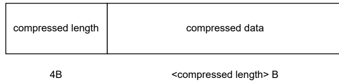
Figure 3.3: The format of the compressed data.
