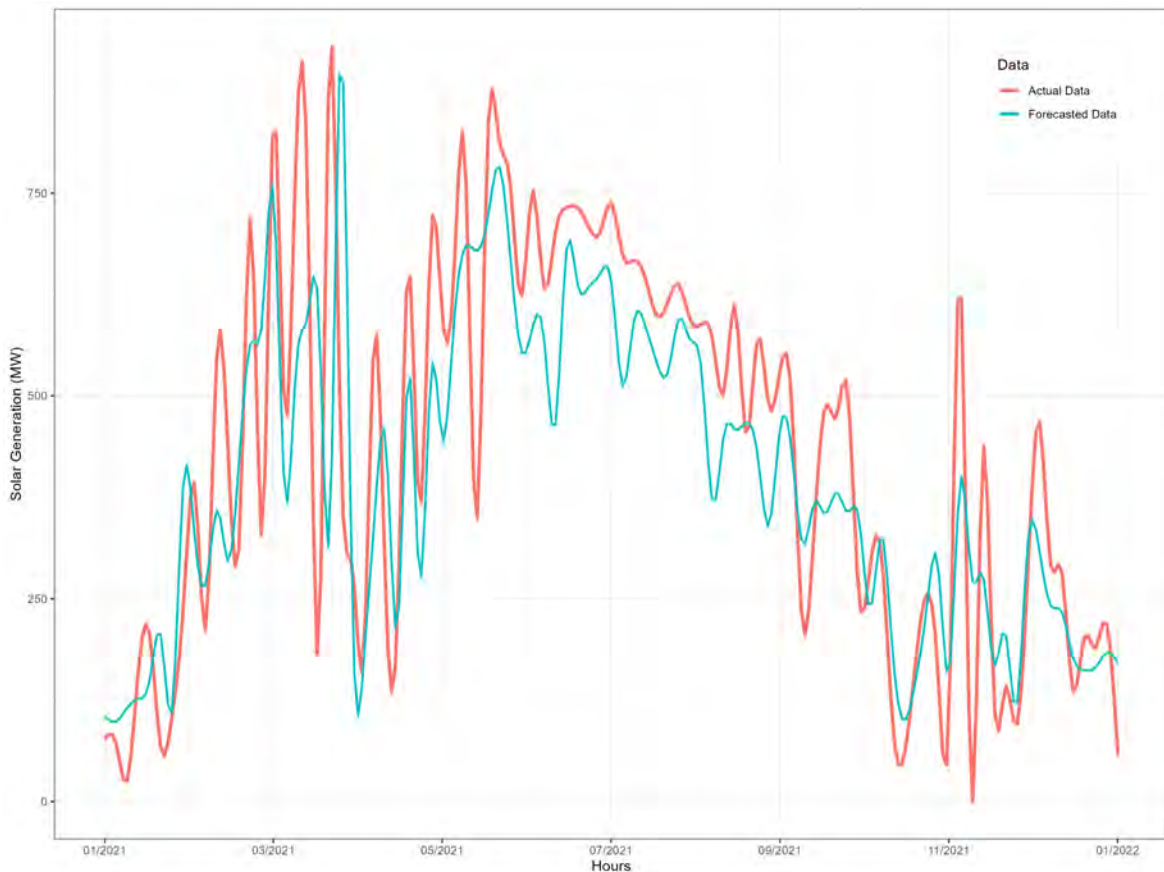
Figure 4.13: Actual and forecasted solar generation based on the model without an FSM.
