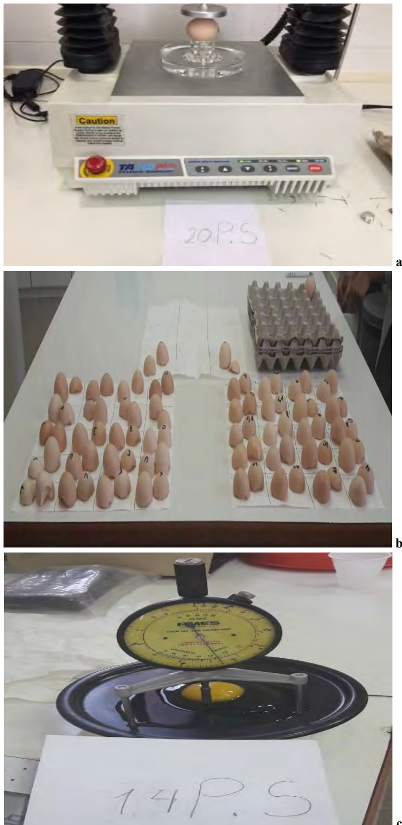
Figure 3 (a, b, c). Evaluation of Egg Quality traits (eggshell strength, shell thickness, albumen height)
