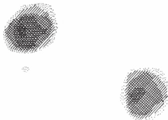
Fig. 2 Proton nuclear magnetic resonance zeugmatogram of the object described in the text, using four relative orientations of object and gradients as diagrammed in Fig. 1.
