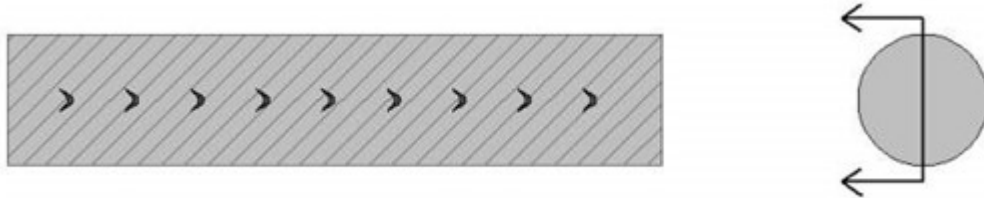
Figure 7: Center cracking in an extruded part (Metal Extrusion. (n.d.))
