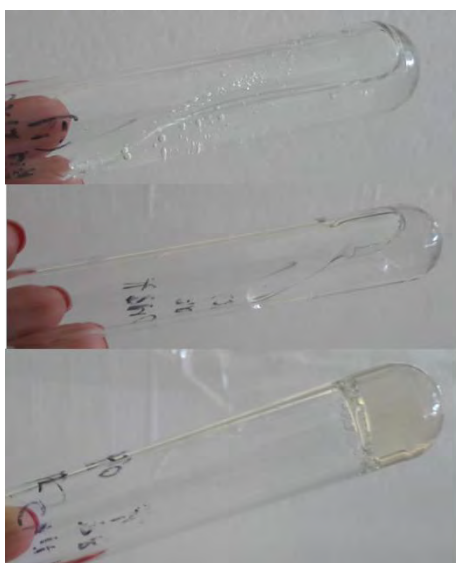
Figure 44. Image from the experimental procedure illustrating the difference in viscosity depending on the polymer concentration in the dispersion medium.
