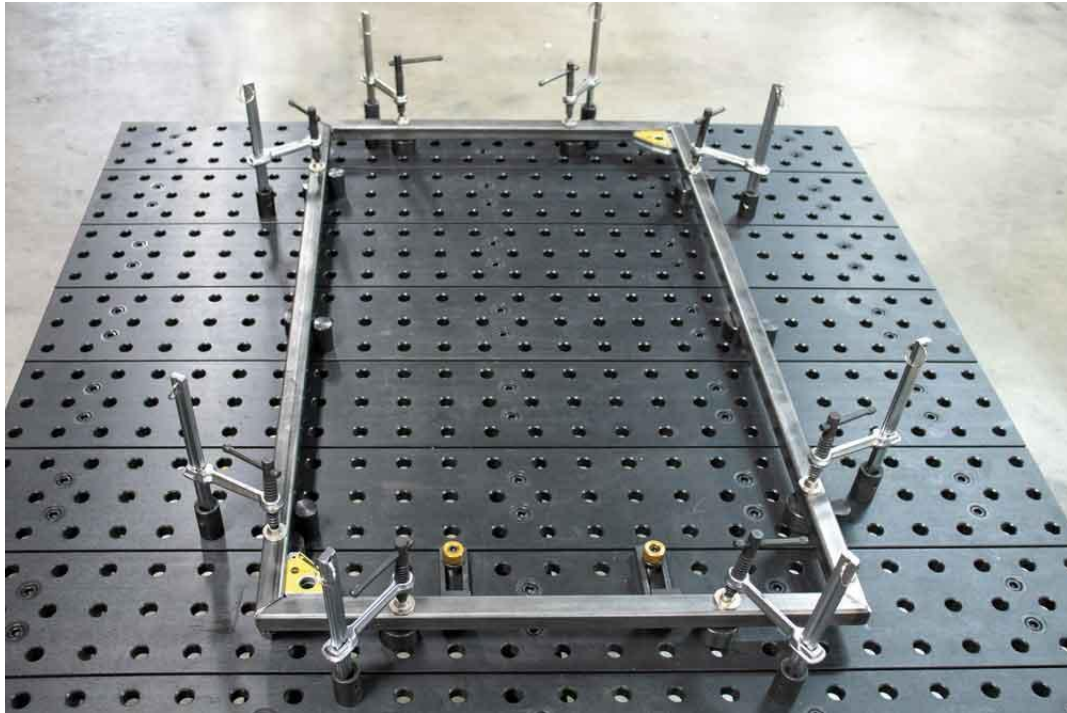
Figure 5.6 Fixturing with jigs [29]
