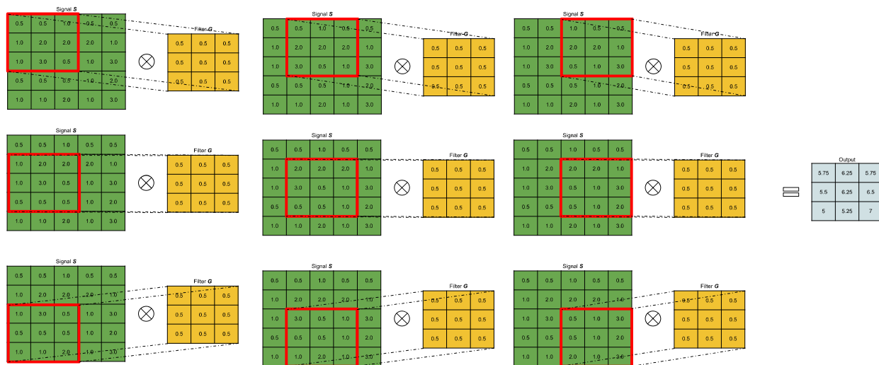
Figure 2.18. Whole convolutional progress along the input signal
