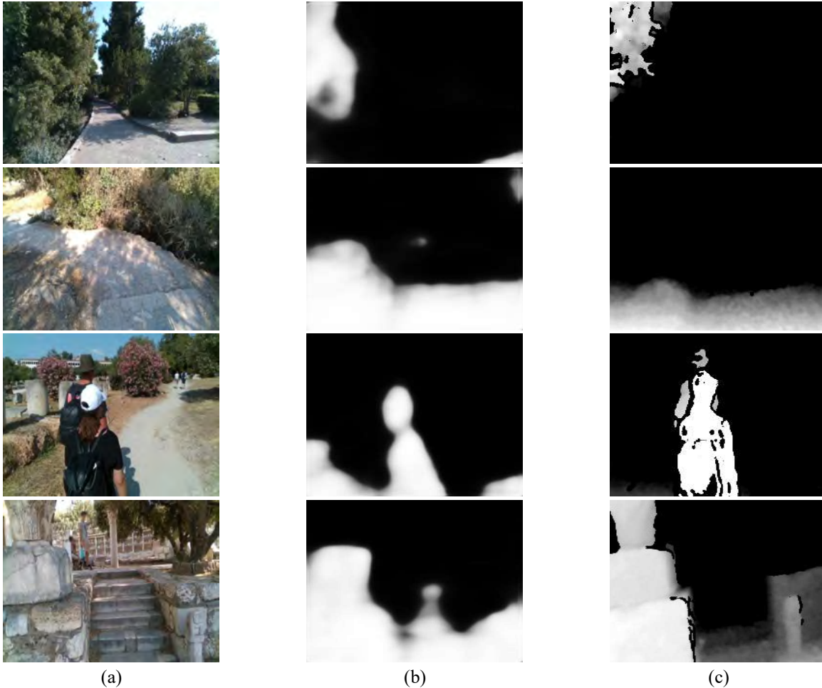
Figure 4.23. Qualitative comparison between the proposed methodology and obstacle maps produced by (George Dimas, Diamantis, et al., 2020), each column represents the (a) input images; (b) Obstacle maps estimated by the proposed model ( O_M^{est} ); (c) Obstacle maps estimated by (George Dimas, Diamantis, et al., 2020) ( O_M^{tr} ).
