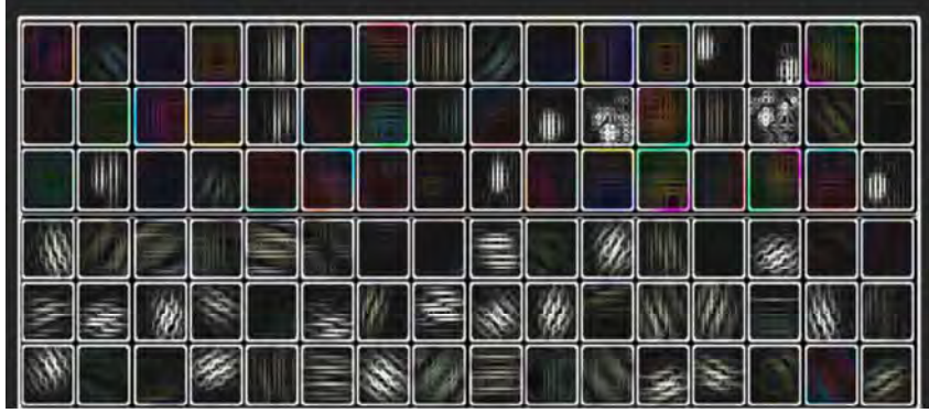
Figure 2.21. Example of trained kernels of a convolutional layer of a CNN model.
