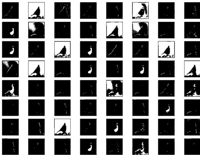
Figure 2.20. Example of feature maps that are estimated by a convolutional layer of a CNN model.
