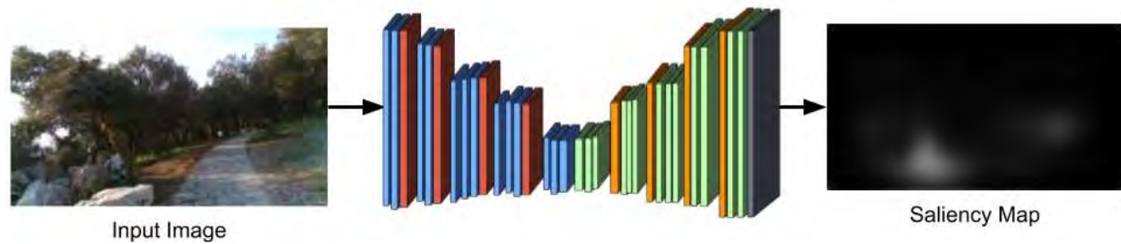
Figure 4.1. Illustration of the SalGAN architecture of the generator.
