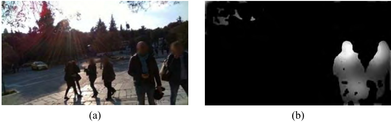
Figure 4.7. Example detection of high-risk obstacles (nearest crowd and tree branches). (a) Original image IRGB. (b) The corresponding image O^1_{obstacle} obtained by using membership function d_l .
