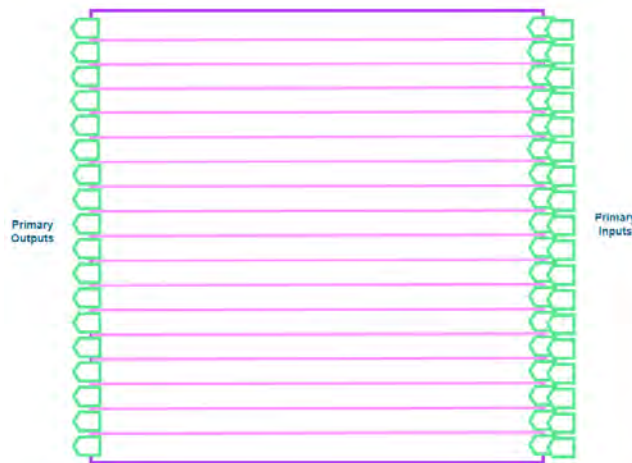
Figure 6.7: Proposed IOs for 33-bit Synthetic Adder
