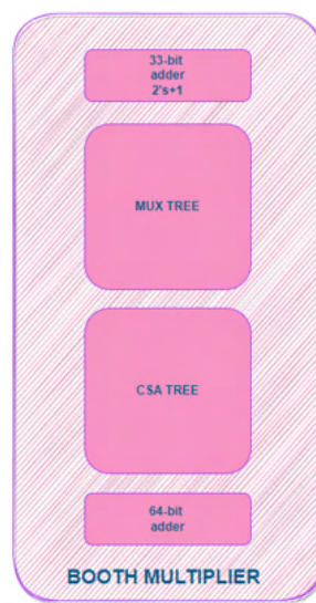
Figure 6.6: Booth Multiplier Block Diagram
