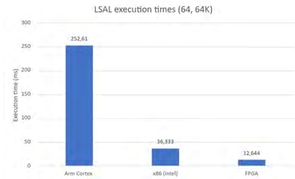
Figure 3.26: Comparison between LSAL execution times across all platforms, for N=64, M=65536
