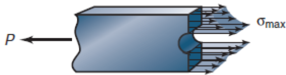
Figure 8 Stress distribution in plate with a hole subjected to axial loading [8]
