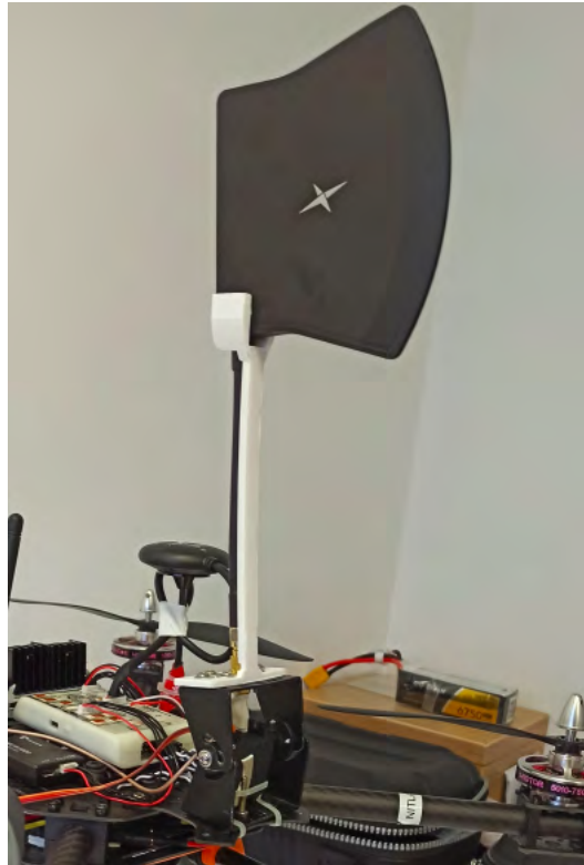
Figure 2.13: Directional Antenna mounted on a UAV
