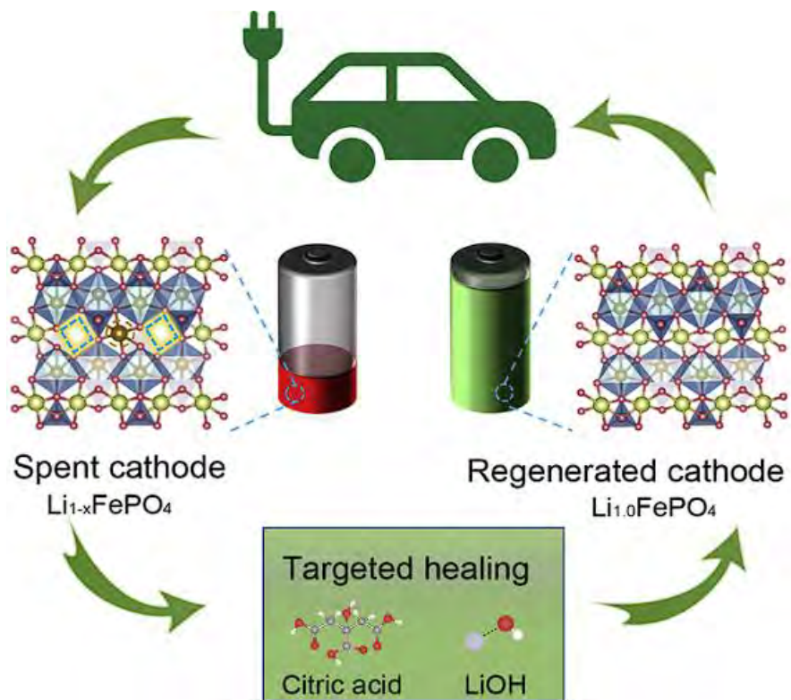
Figure 5.16. The composition, structure, and electrochemical performance of used \text{LiFePO}_4 cathodes with diverse degradation conditions can be entirely recovered to the same levels as those of the pristine materials using a paradigm-shifting lithium-ion battery recycling approach based on defect-targeted healing [378].
