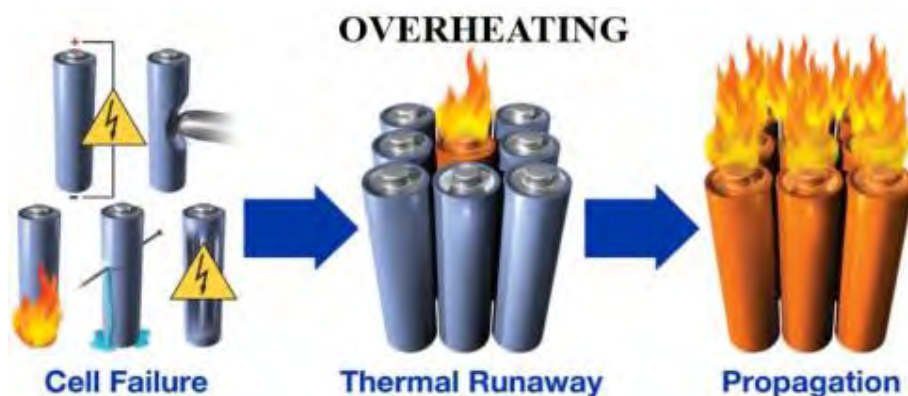
Figure 4.3. Thermal runaway effect on battery [317].
