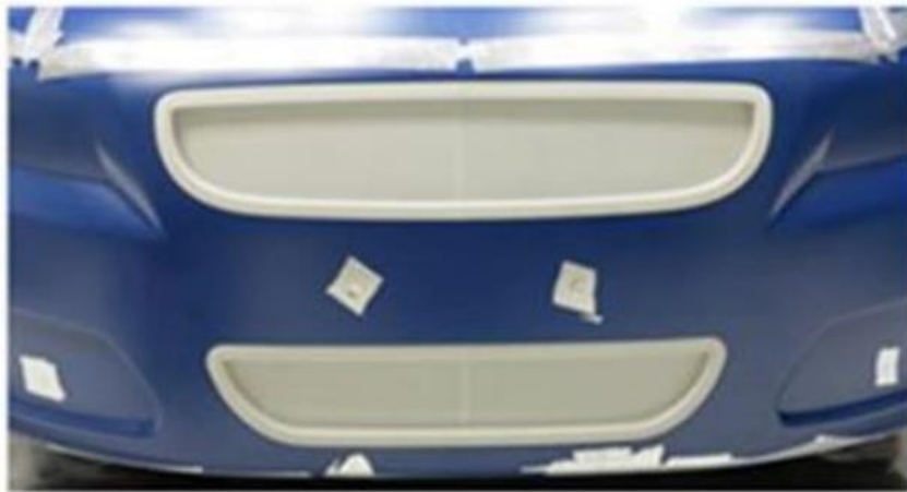
Figure 4: Grill insert based closure of the front grills [1].
