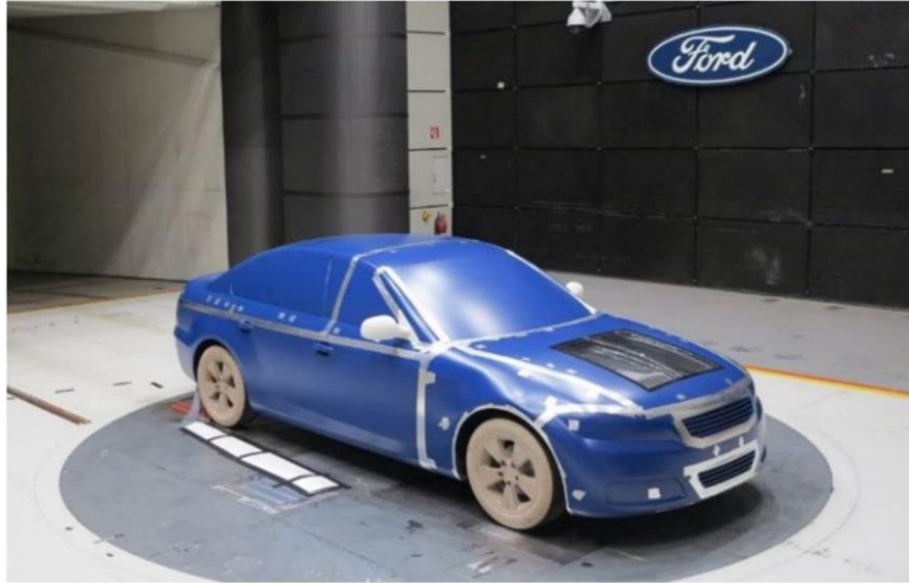
Figure 3: The Ford 1:1 scale notchback Open Cooling DrivAer model [1].
