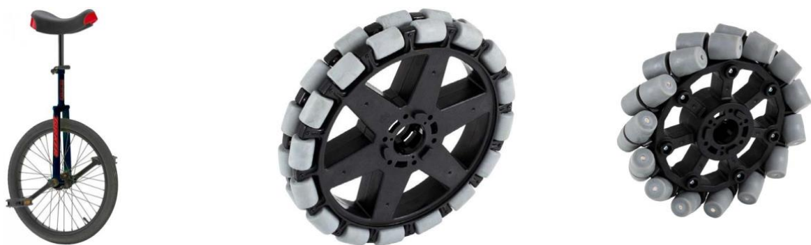
Figure 1.4 (Left) Conventional wheel, (Center) Omniwheel, (Right) Mecanum wheel (Lynch & Park, 2017)
