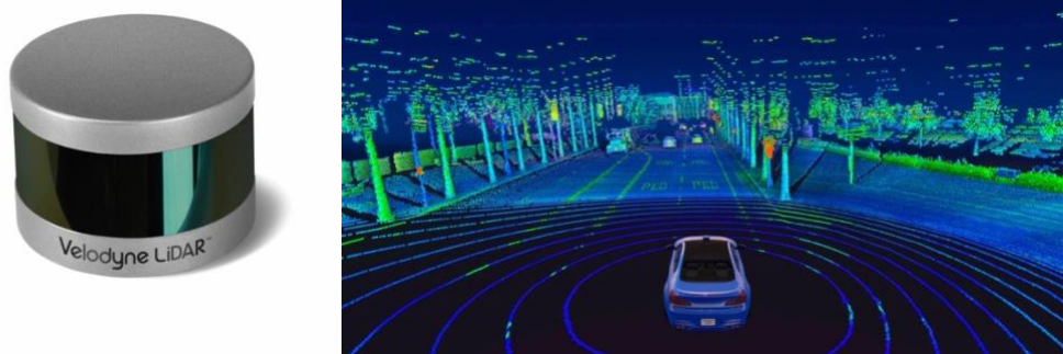
Figure 1.2 A lidar sensor in the left and in the right the result taken from lidar (Velodyne Lidar, 2018)
