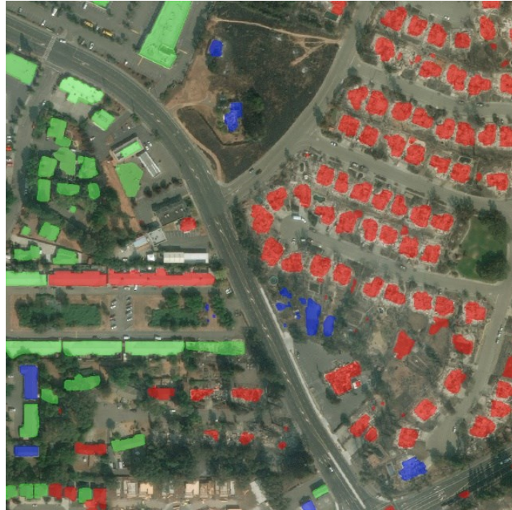
Figure 9 Damage Classification using Non-Linear SVM as last layer (Santa-Rosa-Wildfire)
