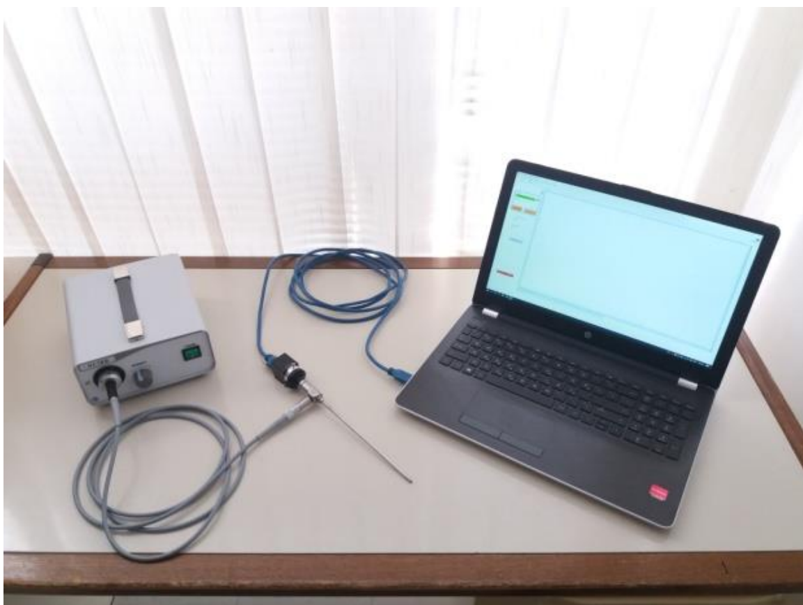
Figure 10. The experimental setup. In this image it is represented the XIMEA multispectral IR sensor, an optical fiber, a light source and connected with a USB3.0 interface cable to a laptop.[33]
