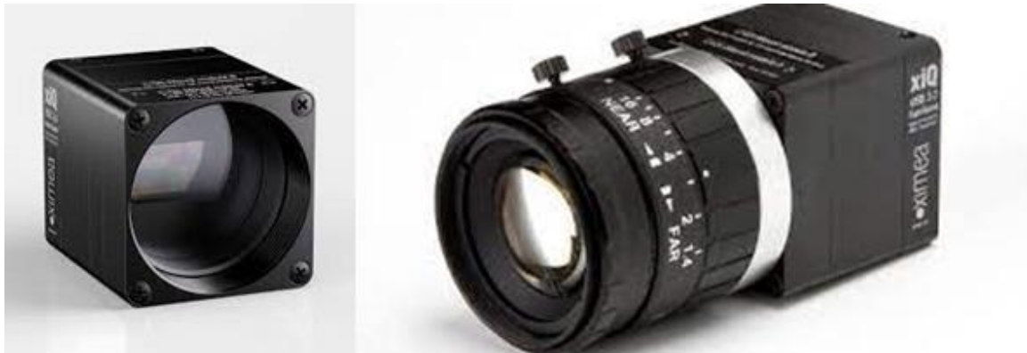
Figure 9. XIMEA camera MQ022HG-IM-SM5X5-NIR. This is the multispectral snapshot camera we used to acquire the data
