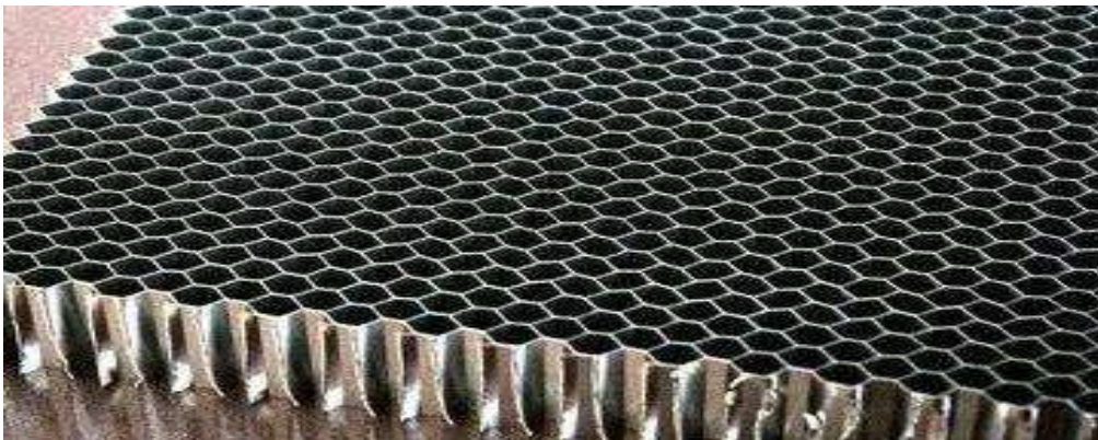
Figure 2.1: Aluminum honeycomb core
