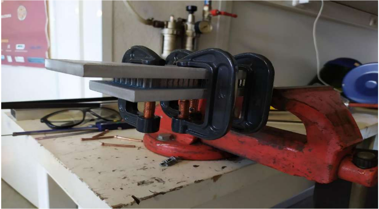
Figure 3.6: Method of tightening the specimen with clamps
