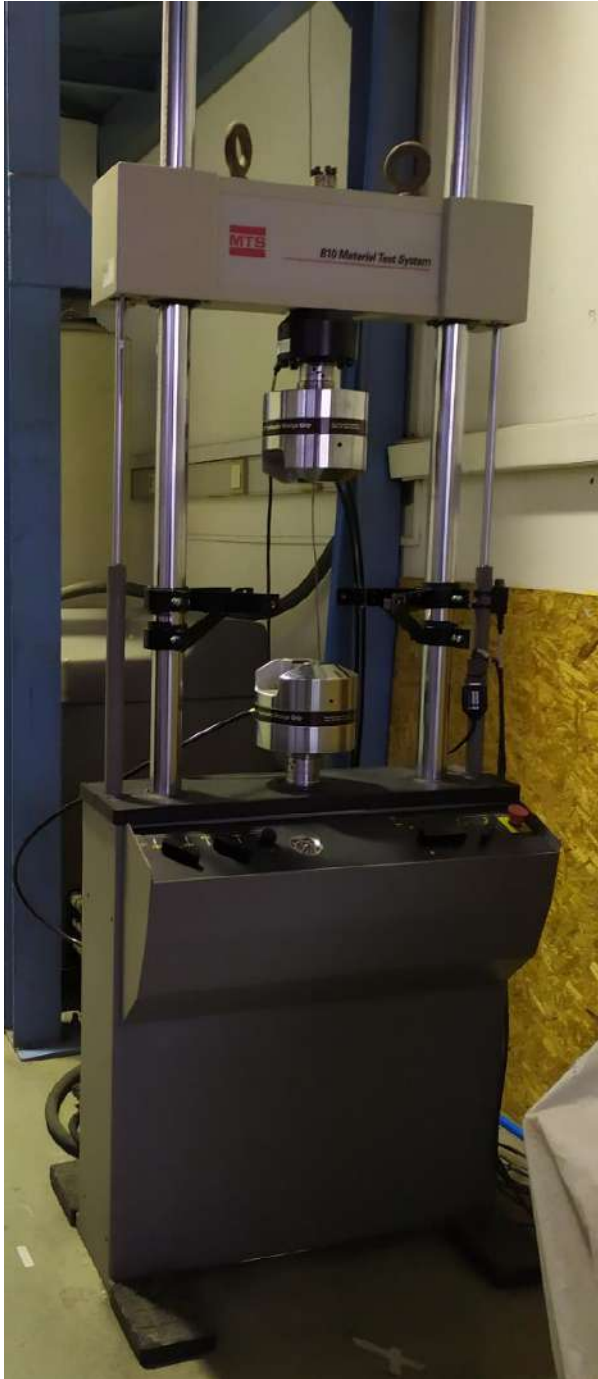
Figure 3.10: (a) MTS 810 Material Test System, (b) Specimen placed upon the MTS system
