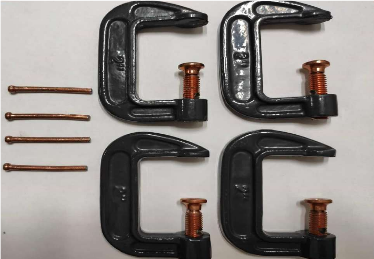
Figure 3.7: Modified clamps for applying pressure at honeycomb specimen and fitting in the mechanical convection oven
