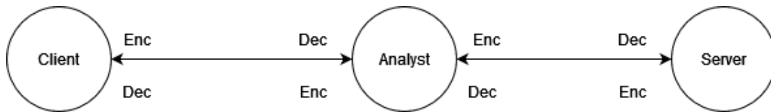
Figure 3.1.1.6 In order for the analyst to perform network analysis in the case of transmission of symmetrically encrypted data, he/she must set himself/herself in man in the middle position between the server and the client decrypting the data flowing in and encrypting flowing out of the controlled node.
