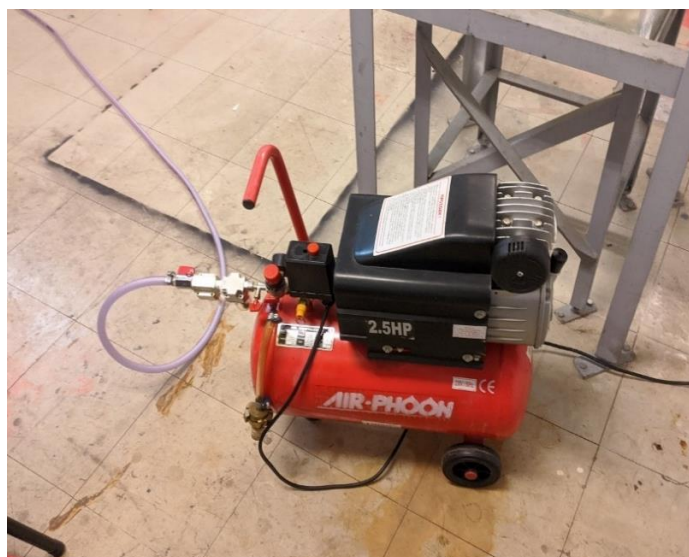
Figure 2-8: The air compressor providing the experimental arrangement with constant supply of air
