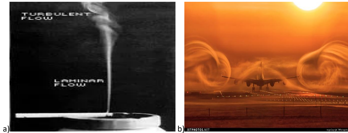
Figure 1-1: Examples of turbulent flow: a) Smoke's flow transition b) An airplane's wake
