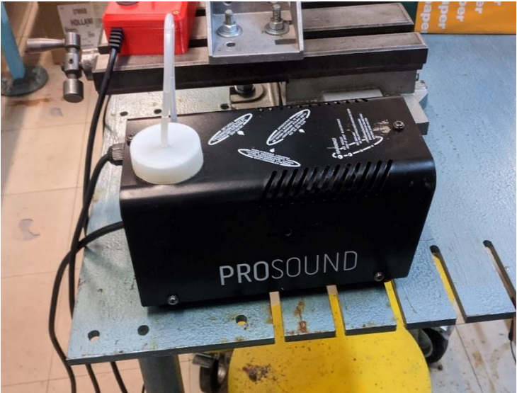
Figure 2-10: The smoke generator used to create the plume
