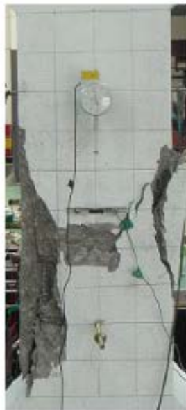
(a) Specimen with natural aggregate, CRC0
