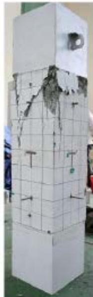
(c) Specimen with natural aggregate, HCRC0
