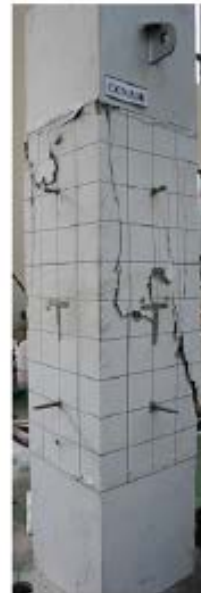
(d) Specimen with mixed recycled coarse aggregate, HCRC30
