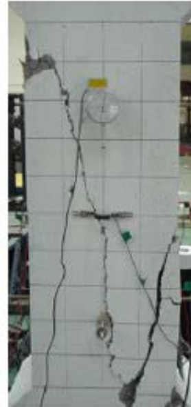
(b) Specimen with recycled coarse aggregate, CRC100
