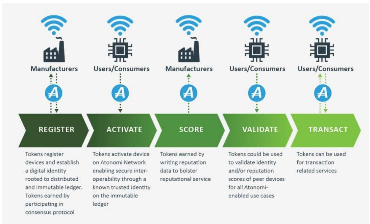
Figure 21: Tokenized IoT Security Ecosystem (Atonomi)
