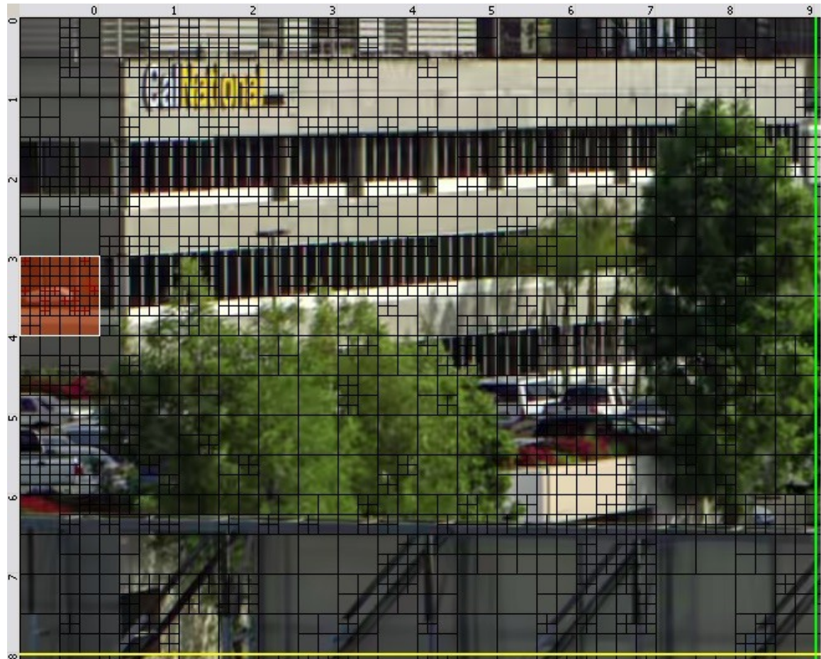
Figure 19: A tile with "dimensions" of 10 x 9 CTUs (green line separates tiles while yellow demarcates slices)
