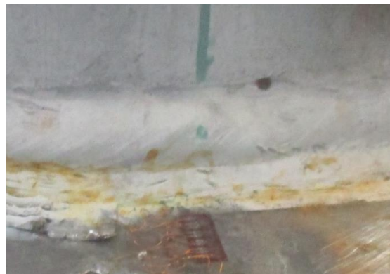
through-thickness crack detail (660,017 cy)
