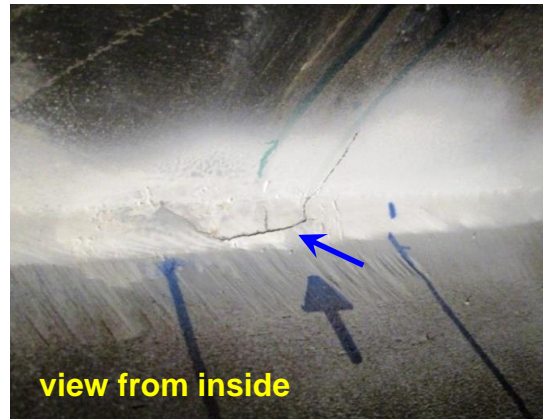
through-thickness crack detail (88,329 cy)
