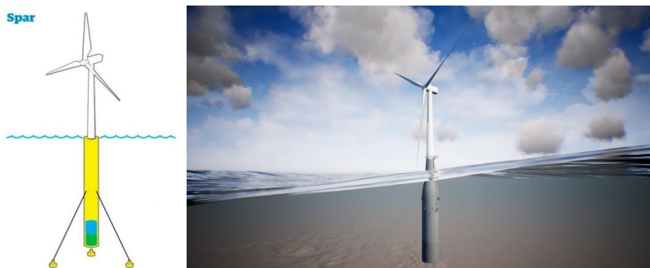
Figure 4: Main design concept of floating spar design wind energy platform (left), Hywind Tampen wind energy platform (right)
