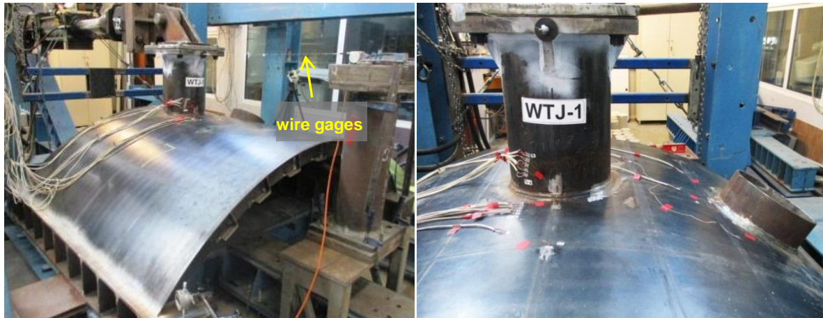
Figure 13: Experimental instrumentation; wire gauge (left) and strain gauges (right)
