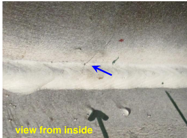
through-thickness crack detail (660,017 cy)
