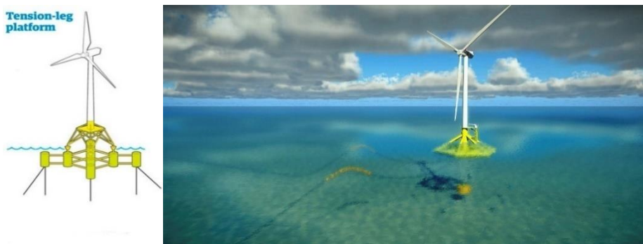
Figure 6: Main design concept of Tension Leg Platform wind energy (left), HEXAFLOAT Tension Leg Platform (right)
