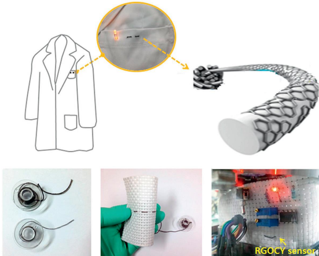
Figure 24: A RGO gas sensor thread with, made of microfiber bundles (cylinders) wrapped with RGO. (B) Cotton and RGO yarns and RGO polyester yarns. (C) Cotton RGO thread gas sensor system sewn on the fabric. (D) The portable gas detection and alarm system. © 2017 University of Cambridge.
