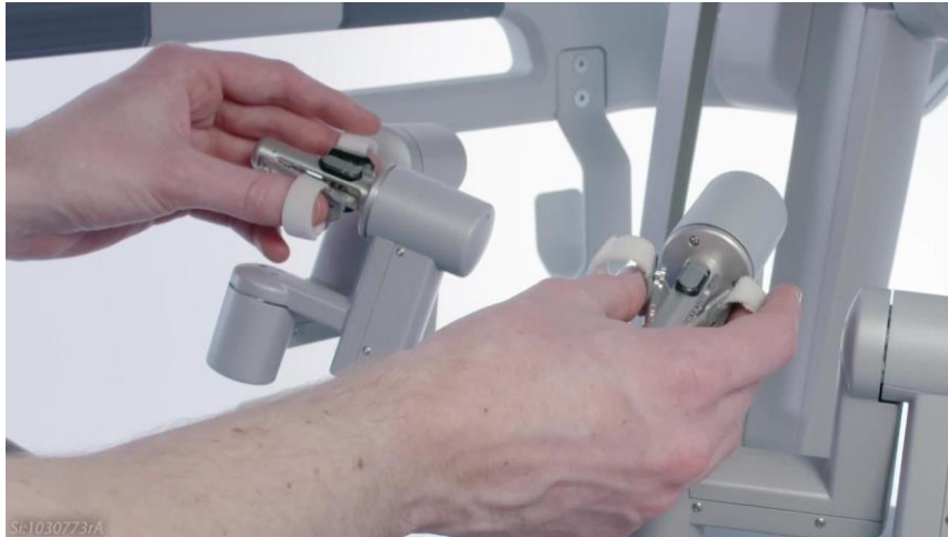
Figure 43: The console of a robot assisting in laparoscopic surgery. © 2021 Intuitive Surgical, Inc.
