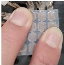
Fig. 3. Structure of the silicone rubber covering the pressure sensitive part (Four layers of silicone rubber sheets with different elasticities are utilized for positioning and upgrading the pressure sensitive part.)
