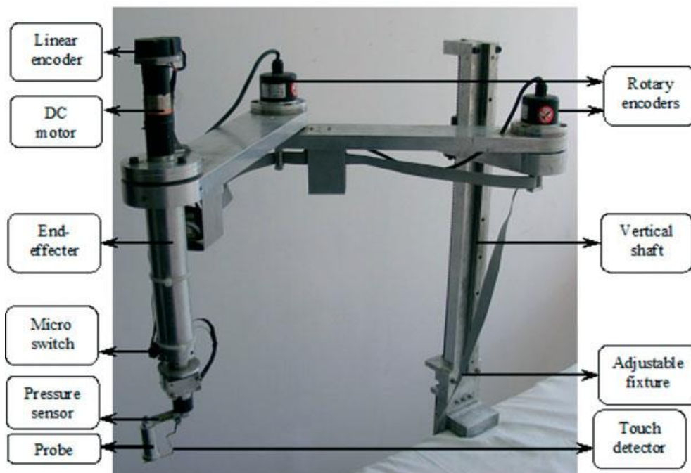
Figure 11: The Robo-Tac-BMI and its parts (© 2011 John Wiley & Sons, Ltd.)
