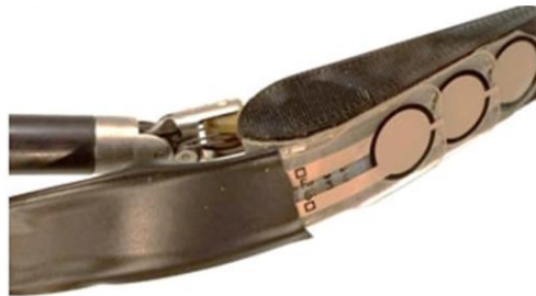
Figure 9: The sensors mounted on the forceps of the robotic arm. © 2019 Springer Nature Limited.
