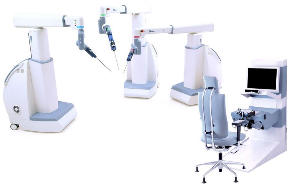
Figure 2: The Senhance surgical robot with its three arms and console. © 2021 Asensus Surgical US, Inc.
