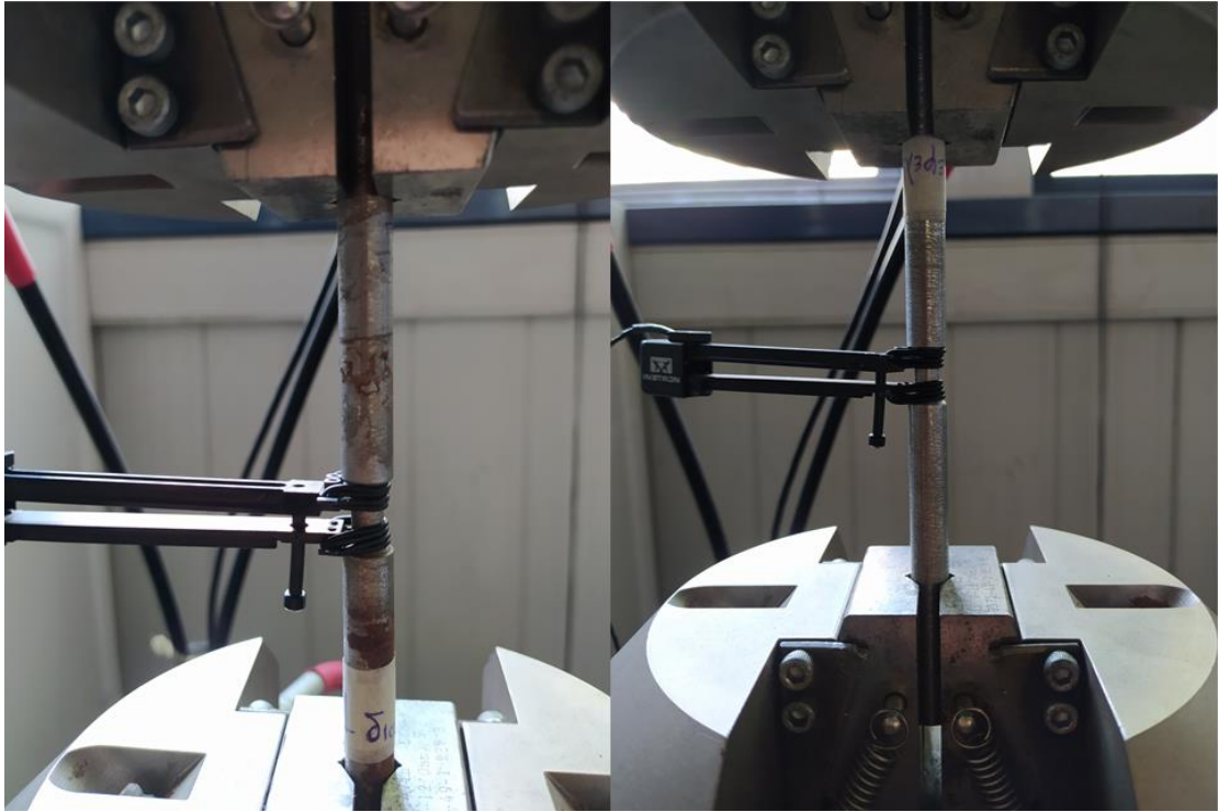
Figure 5.4 Corroded and new specimen tensile tests
