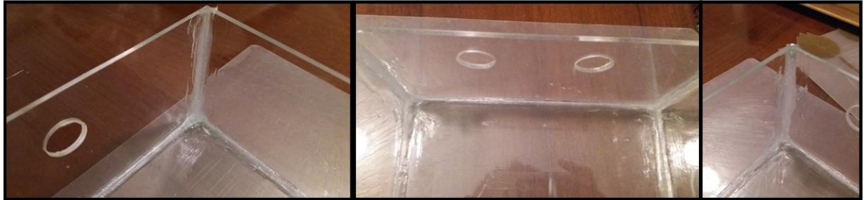
Figure 4.2.1.7 Application of silicone on the edges
