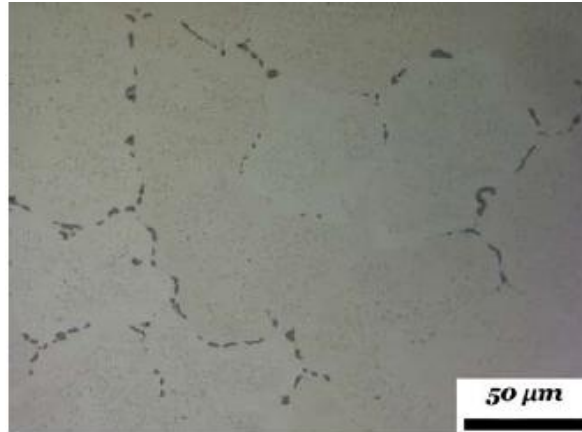
Figure 4: metallographic images of Alloy 6060: a) as-cast microstructure, homogenized at 560°C b) for 4 hours and c) for 6 hours.
