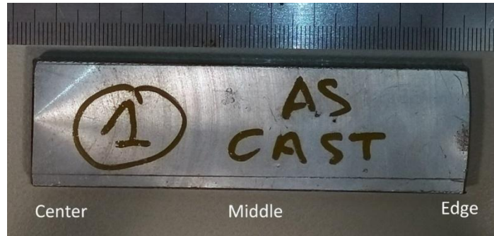
Figure 16: As-cast Al-alloy 6060, sections of received as-cast for the characterization analysis.
