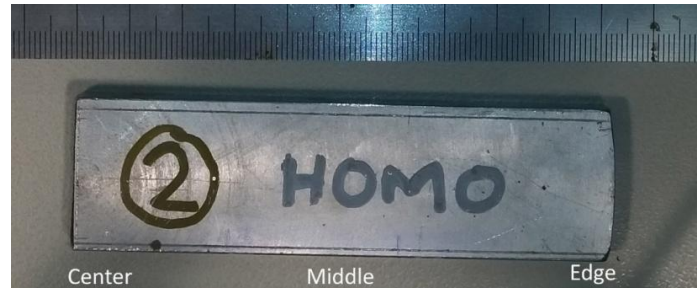
Figure 21: As-homogenized Al-alloy 6060, sections of received as-homogenized for the characterization analysis.
