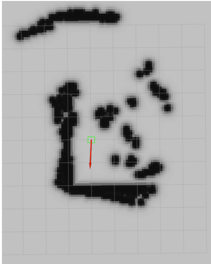
Figure 4.3 Global cost map. Black cells are inflated objects, green rectangle is the robot and the red arrow represents its orientation.
