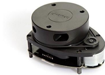
Figure 2.7 RPLidar A1M8 device.
