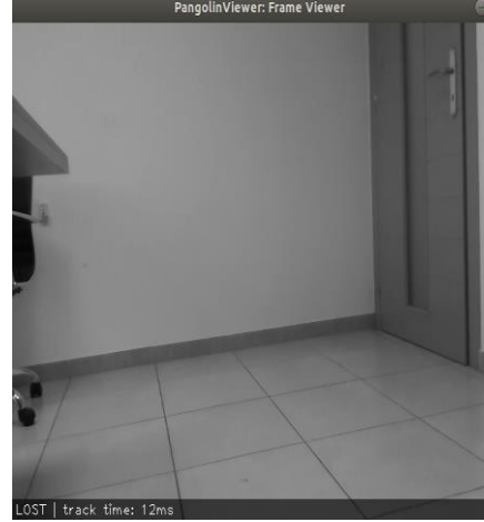
Figure 5.13 The chair is moved out of the field of view, camera is back on the starting position and the algorithm is still lost.
