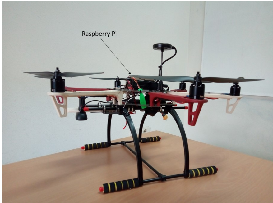
Figure 4.1: Custom polycopter of our lab with a Raspberry Pi as a companion board
