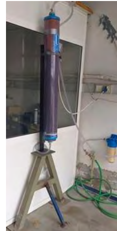
Figure 4-8: The deionizing column.
