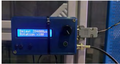
Figure 4-3: The Arduino microcontroller-LCD Keypad system showing regulating the wanted capturing delay.
