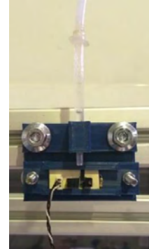
Figure 4-4: Droplets crossing the photo interrupter (black).
