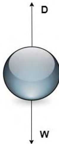
Figure 4-9: Forces acting on a free-falling drop under air resistance effects.
