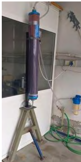
Figure 4-5: The deionizing column.
