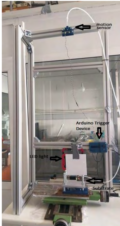
Figure 4-2: Drop impact aluminum support structure.
