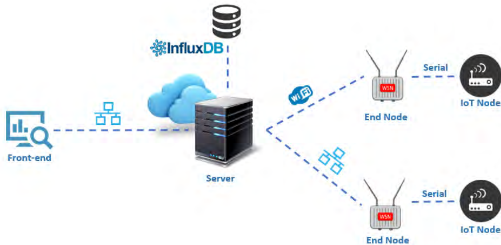
FIGURE 3.5: Remote control architecture
