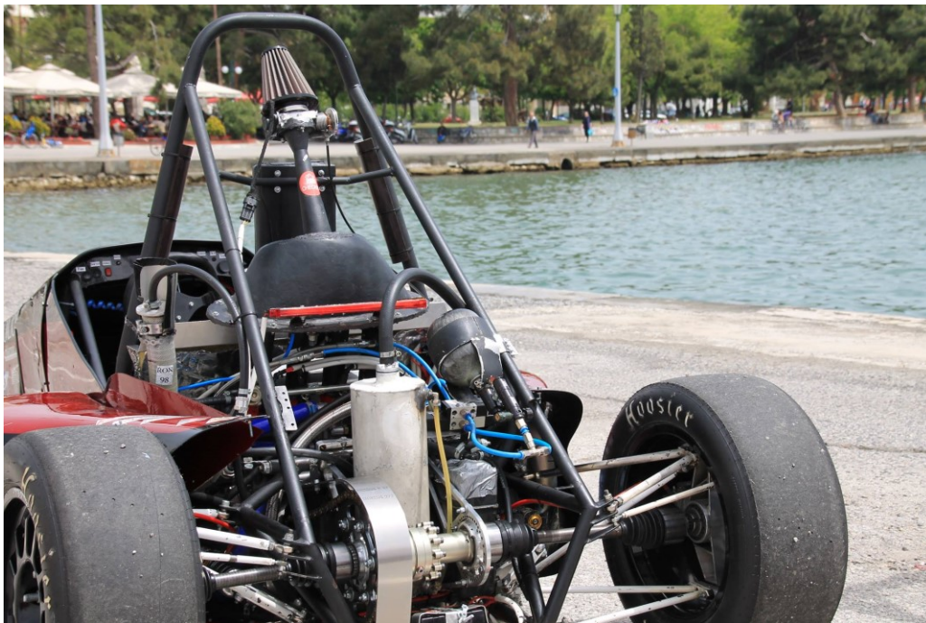
Figure 57 - Back view of Thireus featuring the air intake system
