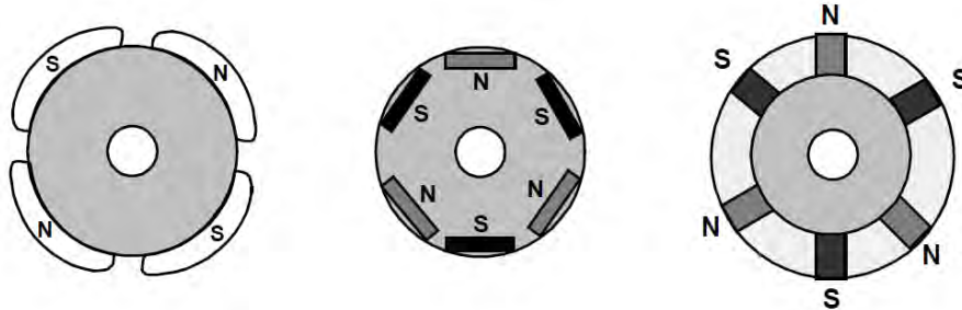
Figure 2.7 In the first rotor the magnets are placed on the surface of the rotor, in the second the magnets are embedded horizontally in the rotor, and in the third they are placed vertically
