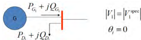
FIGURE 3.4: A slack bus. (Image adapted from [12])
