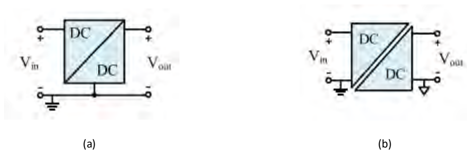
Figure 3. 2 (a) Structure of non-isolated DC/DC converter, (b) Structure of isolated DC/DC converter [1]
