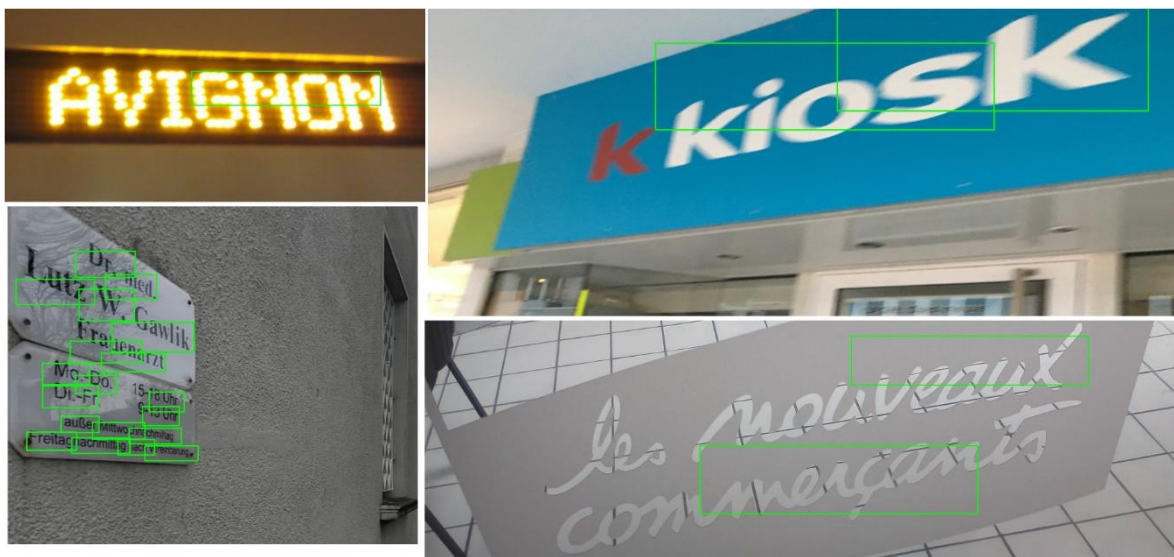
Figure 27. Cases where the text detector fails to cover the whole word with the bounding box.
