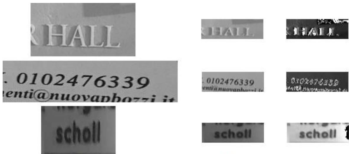
Figure 23. The cropped image goes through three stages before it is given as input to the CRNN. a.. Grayscale. b. Resize to 32 x 100 pixels. c. Normalization to [0, 1].
