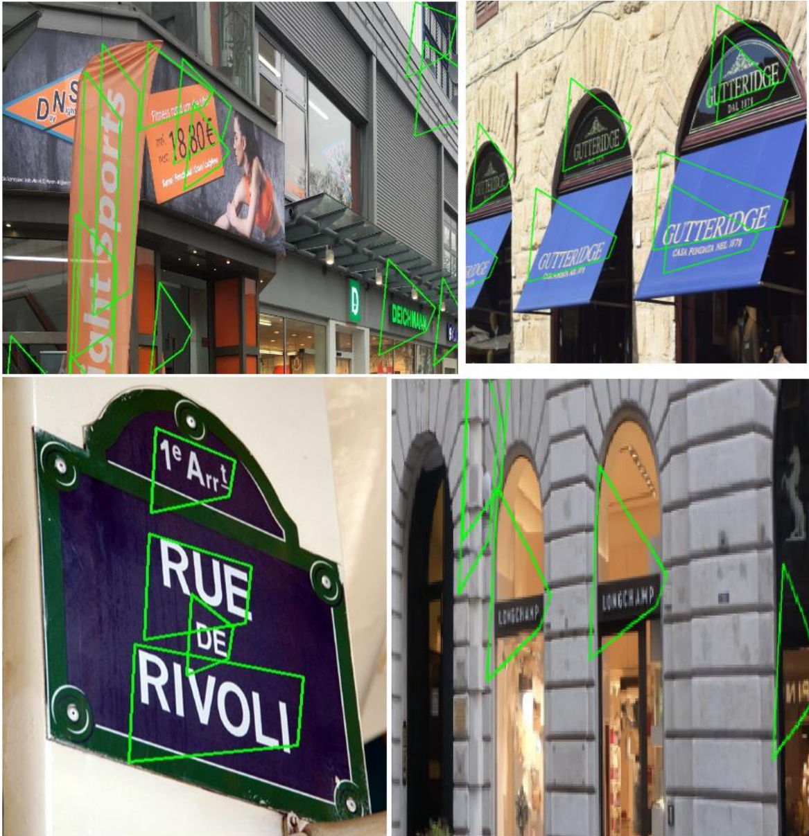
Figure 10. In the cases of diagonal text, shown in Figure 9, we propose this trapezoid bounding box.
