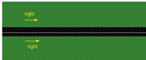
Figure 5.1: SUMO instance for the first network that consists of 2 parallel right-way roads. The first road includes 3 lanes while the second one includes 2 lanes.
