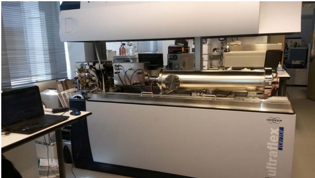
Figure II.9. Views of the MALDI-TOF mass spectrometre.
