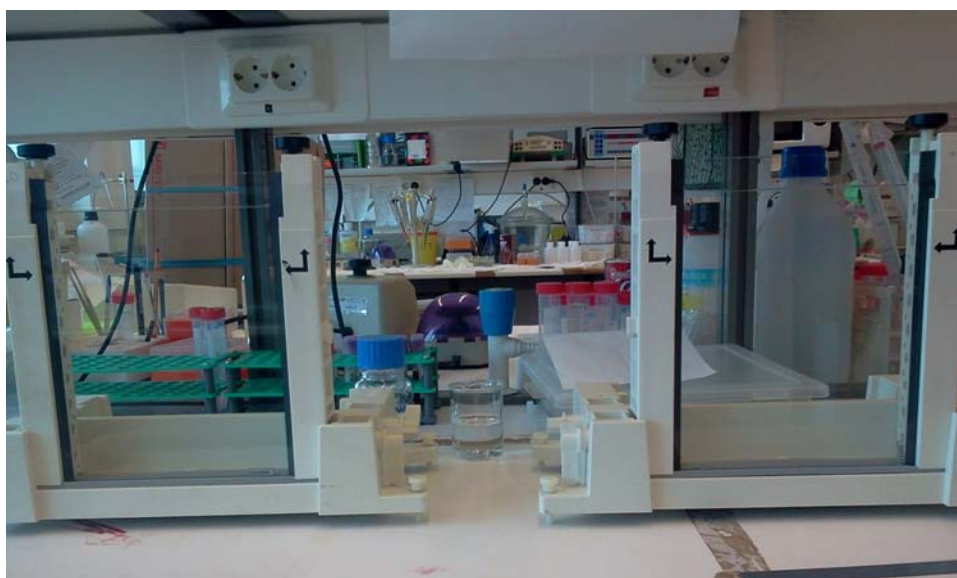
Figure II.4. Two 'cassettes' plugged into respective assembly stations, filled with distilled water, in order to check for possible presence of leaks therein.
