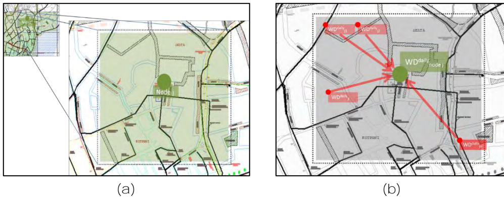
Figure 27. (a) Each node will be a node of the hydraulic model that will be used to estimate the pressure map out of the water demand map. (b) Each node serves a billed consumption that comes out by adding the household billed consumptions that are supplied by the specific node of the network.
