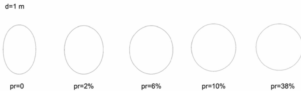
Figure 5.24: Evolution of cross-sectional deformation in pressurized pipelines for the same fault displacement d = 1\text{ m} (X65 steel, D/t = 96 , Clay I, \beta = 25^\circ ).
