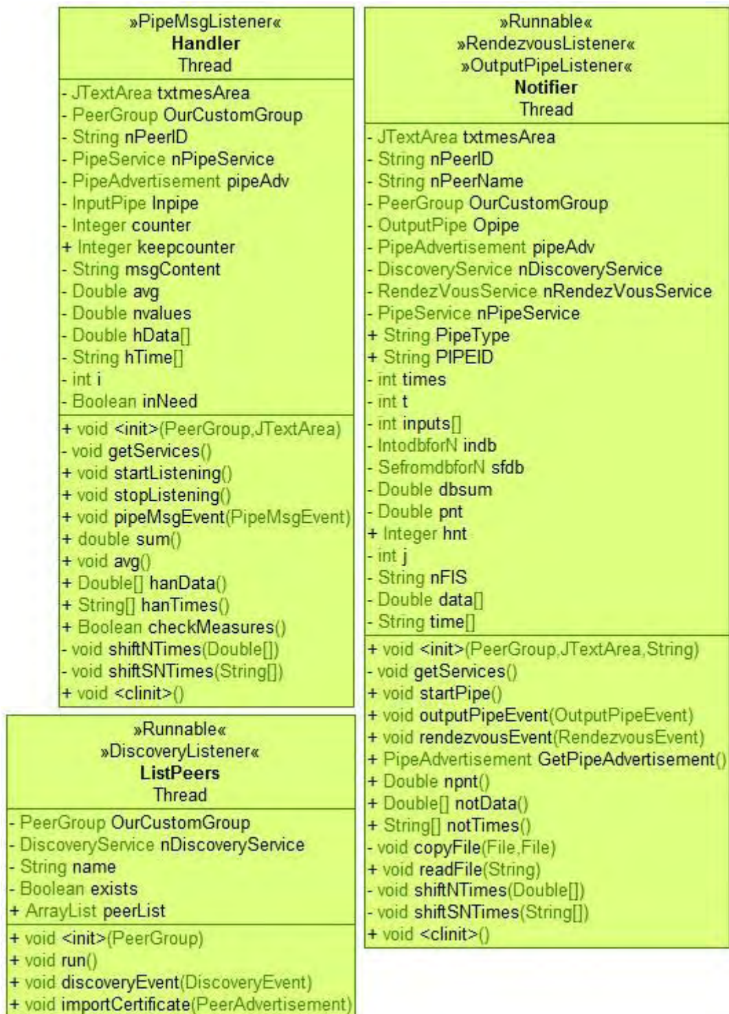
Figure 4.4: UML diagrams of Handler, Notifier, ListPeers
