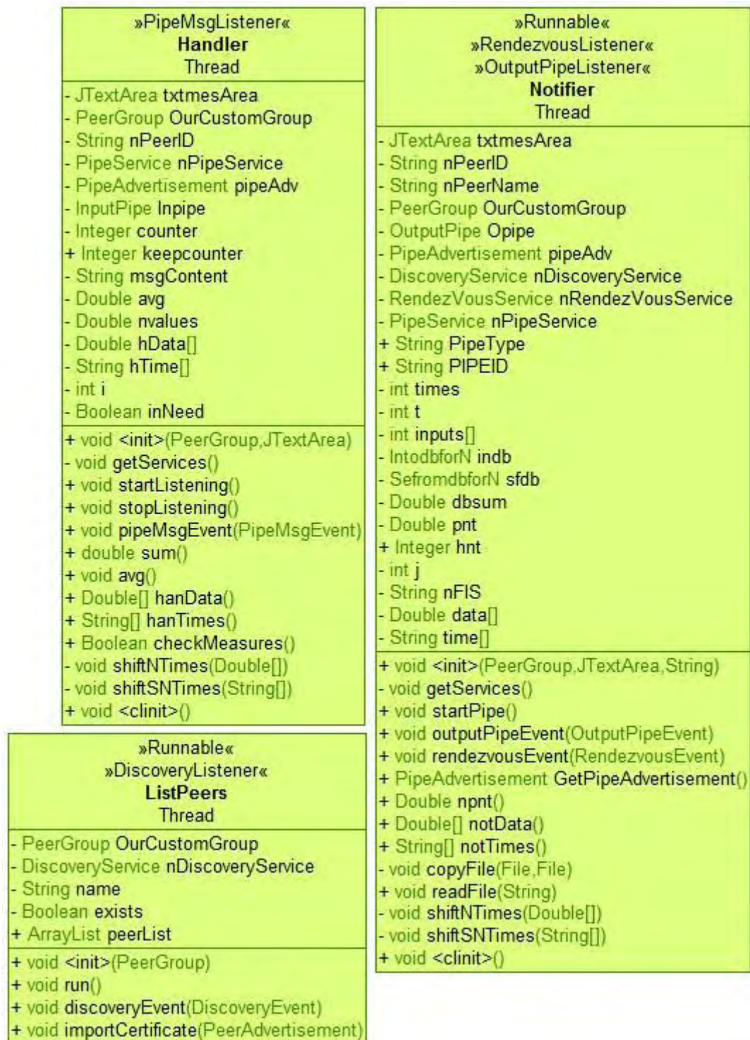
Figure 4.4: UML diagrams of Handler, Notifier, ListPeers
