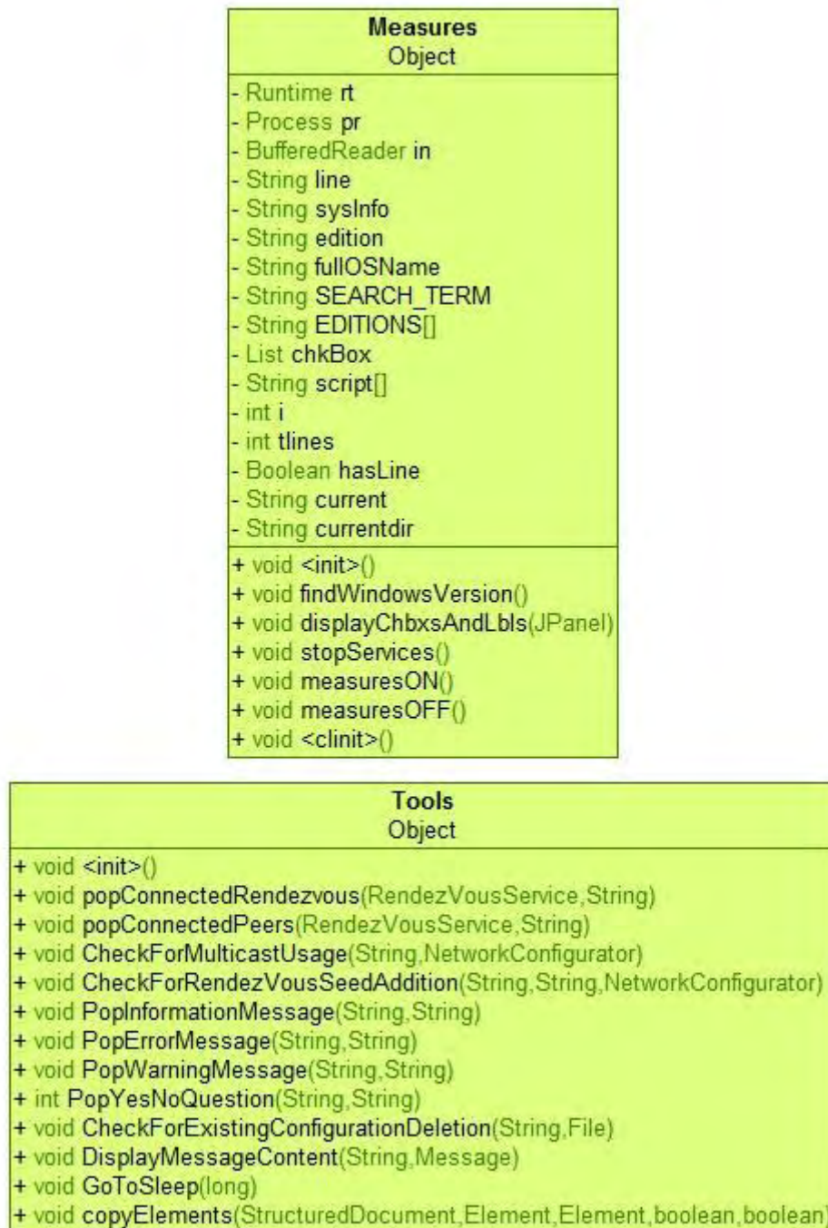
Figure 4.7: UML diagrams of Measures, Tools
