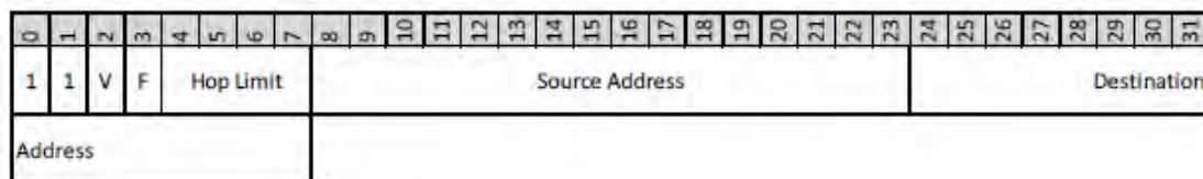
Figure 23: Mesh addressing header of 6LoWPAN
