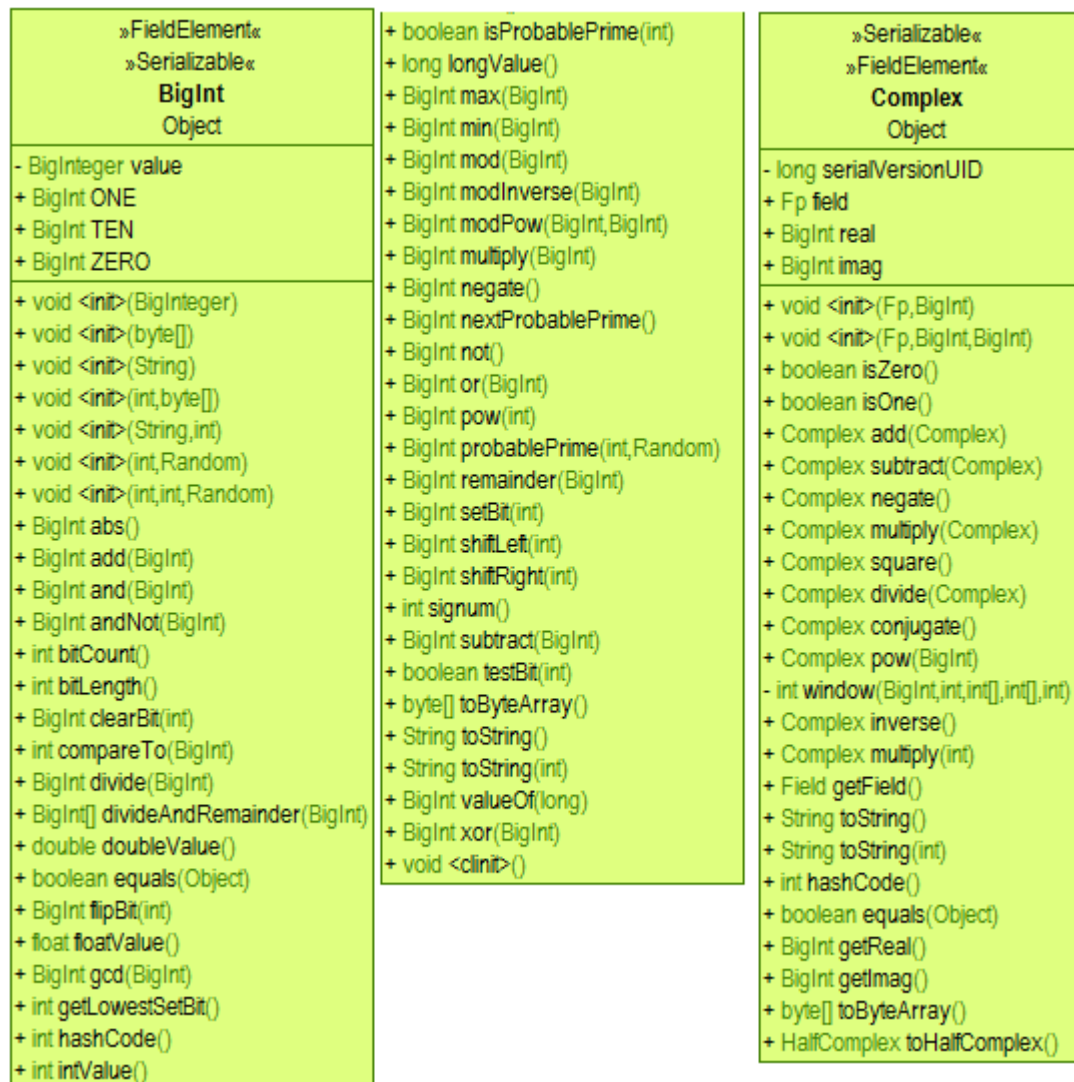
Figure 3.2: UML diagrams of BigInt and Complex classes
