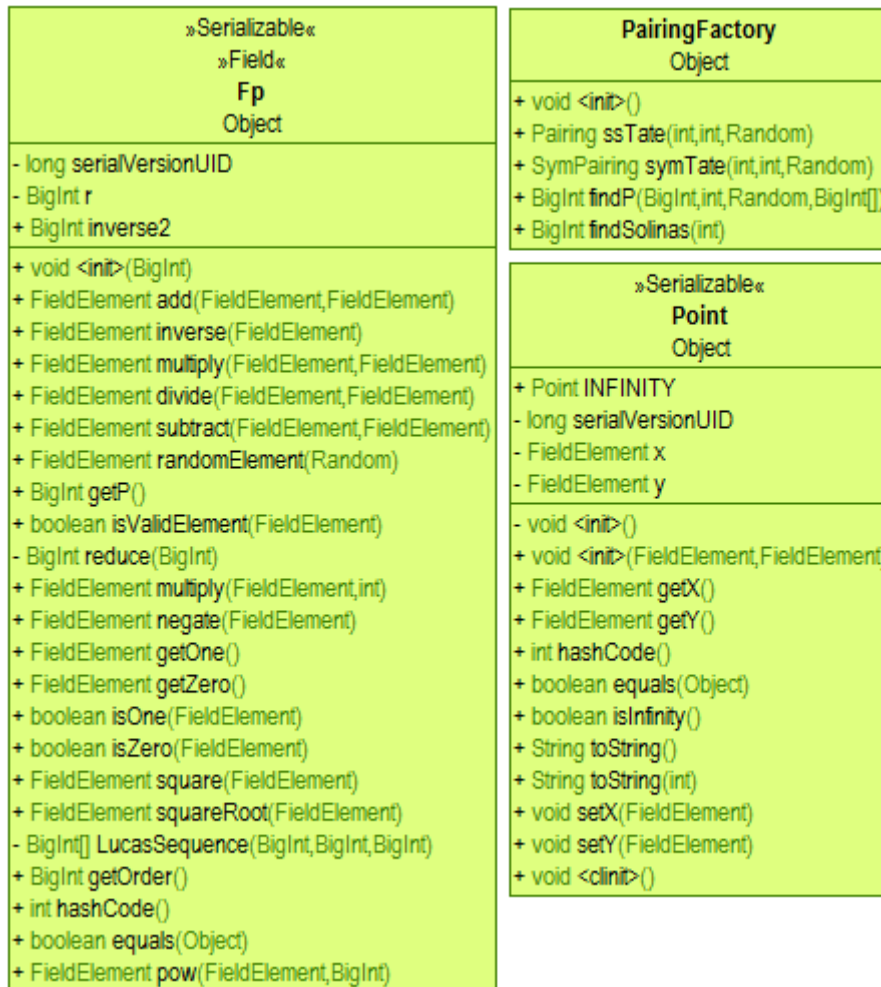
Figure 3.5: UML diagrams of Fp, PairingFactory and Point classes
