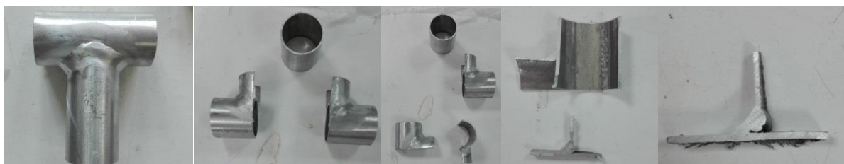
Figure 8: Cutting sequence of the 7005 T1-T1 and T6-T6 welded pipes.
