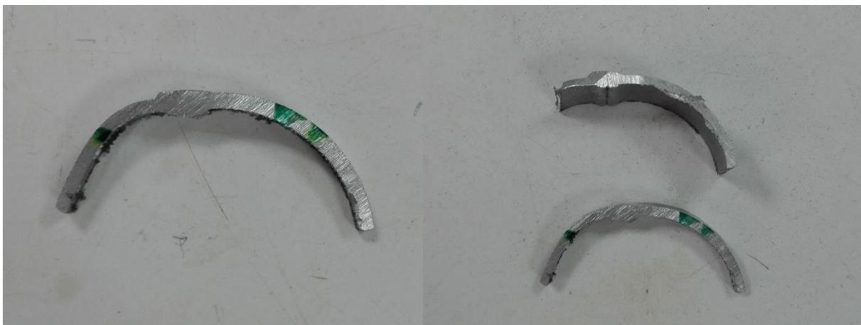
Figure 18: Samples of the T1-T6 welding. Half-cylindrical samples created by cutting the above plate vertically to the welding.
