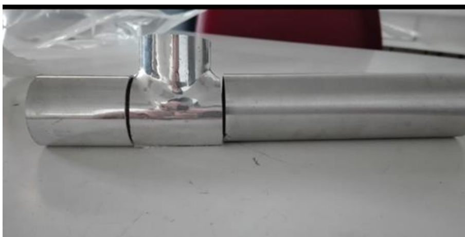
Figure 6: Photograph of the welded T1-T1 pipes.
