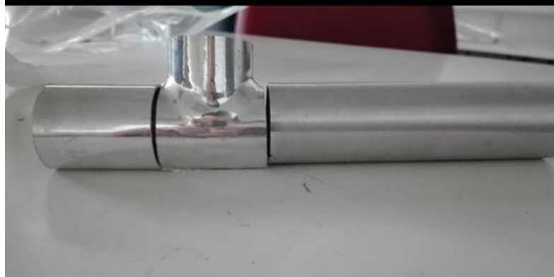
Figure 27: Macrograph of MIG welding between the 7005-T1 pipes.
