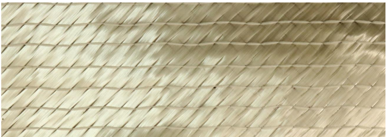
Figure 9– Image – The biaxial side of a triaxial fiberglass fabric
