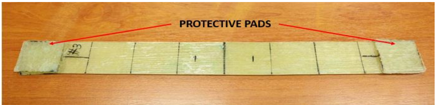
Figure 16 – Image – Tensile specimen with a stepped repair
