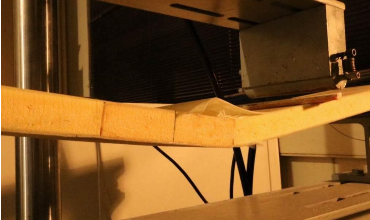
Figure 24 – Image – Failure of specimen with stepped 20mm overlap repair in the compression side
