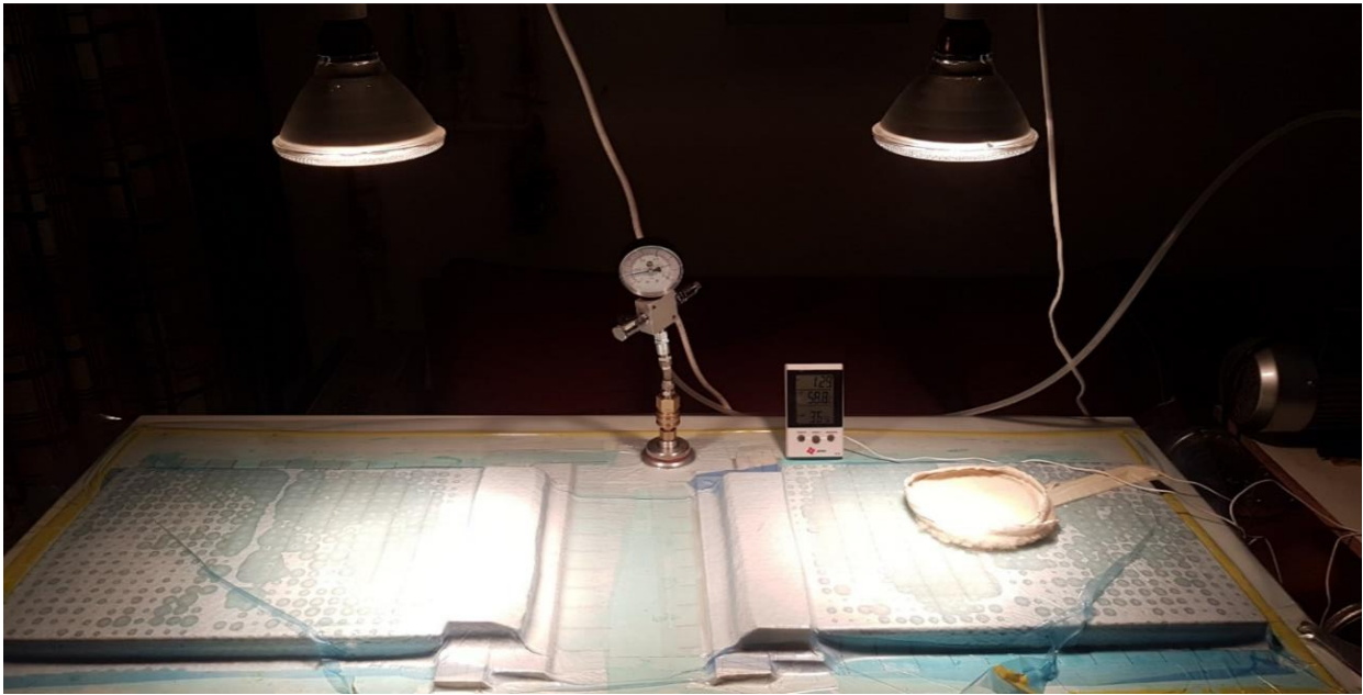
Figure 11 – Image – Ongoing vacuum-curing procedure after the impregnation of the fiberglass fabrics
