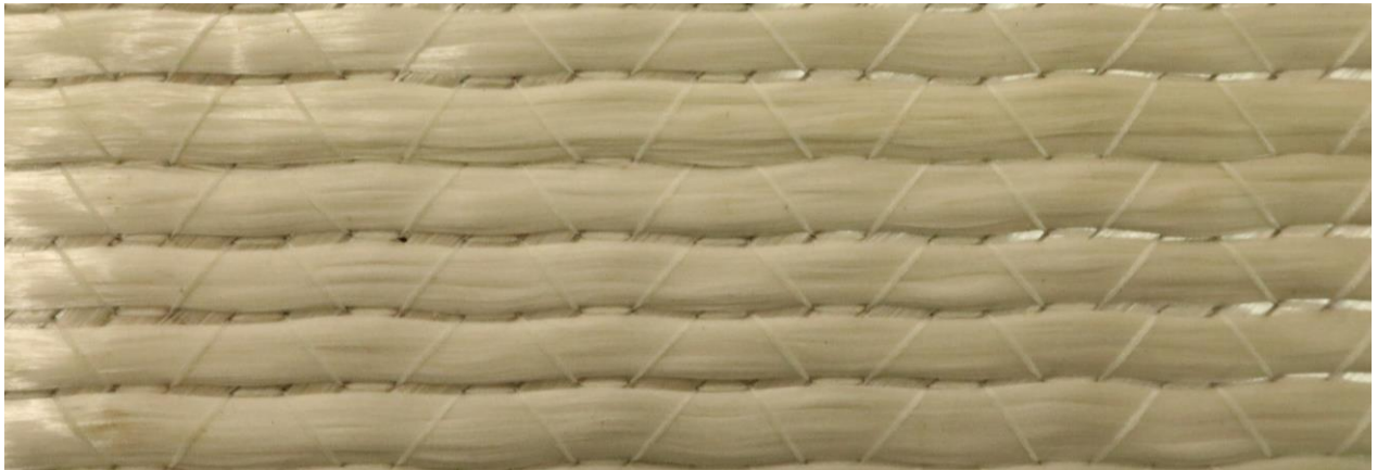
Figure 8– Image – The unidirectional side of a triaxial fiberglass fabric
