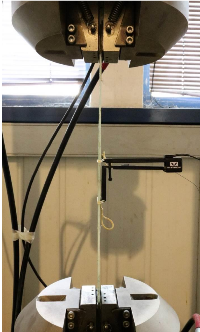
Figure 21 – Image – Tensile experimental set up
