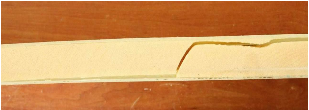
Figure 44 – Image – Four-point bending specimen without repair in its structure- Delamination failure mechanism
