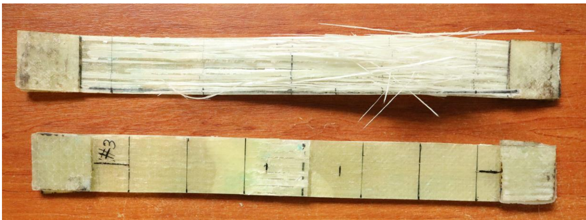
Figure 47– Image – Repaired and non-repaired Tensile specimens after failure
