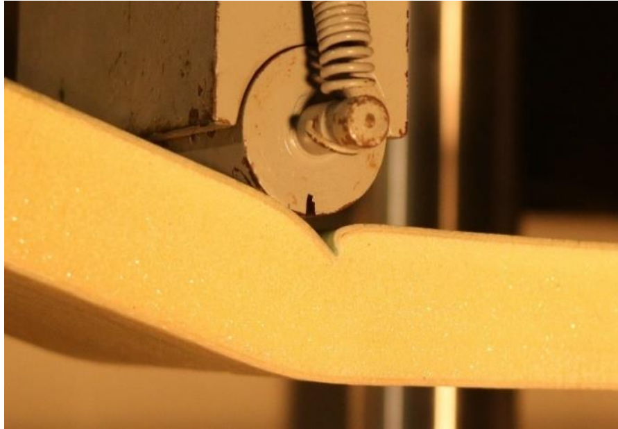
Figure 22 – Image – Failure of specimen tested without pads
