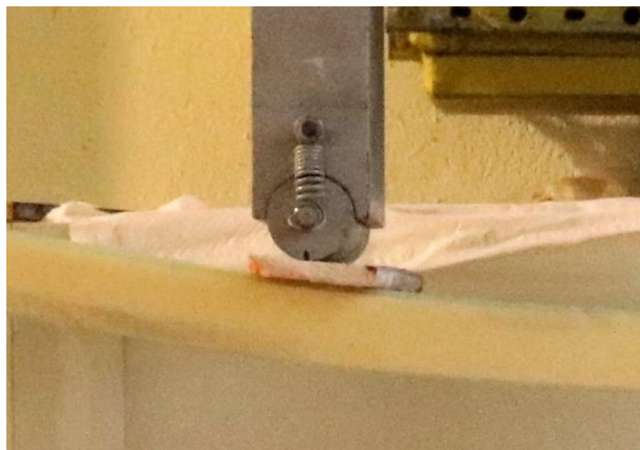
Figure 23 – Image – Testing of specimen with the use of pads
