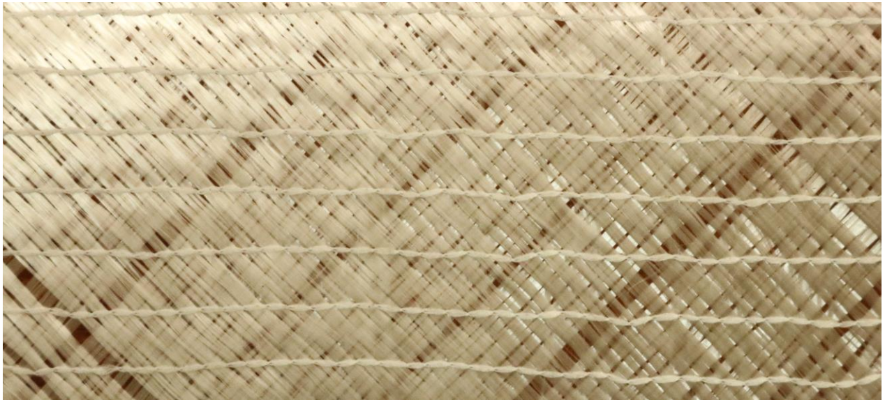
Figure 7– Image – Biaxial fiberglass fabric
