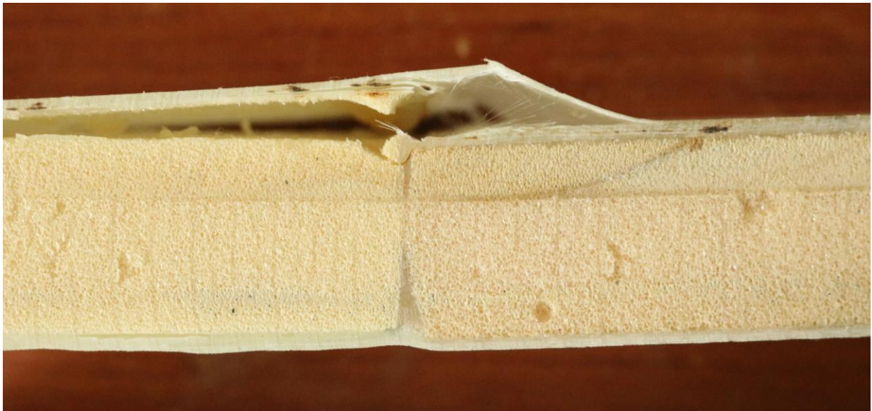
Figure 43 – Image – Four-point bending specimen with stepped repair in its structure – Delamination failure mechanism and fiber breakage
