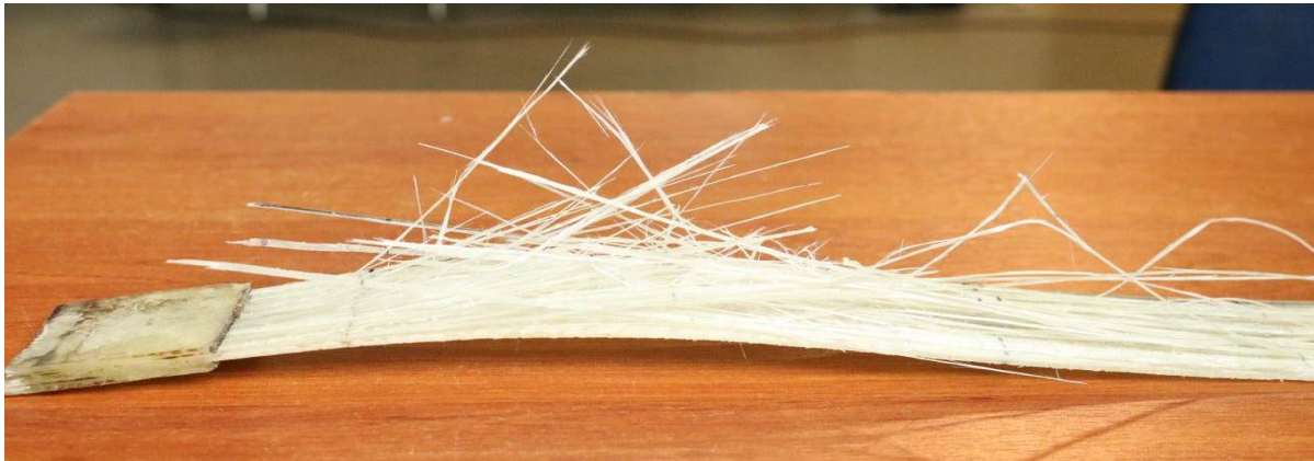
Figure 46 – Image –Tensile specimen with no repair in its structure – Matrix and fiber failure
