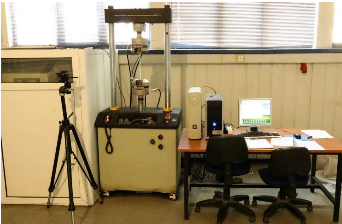
Figure 17 – Image – Tensile machine Instron 8801
