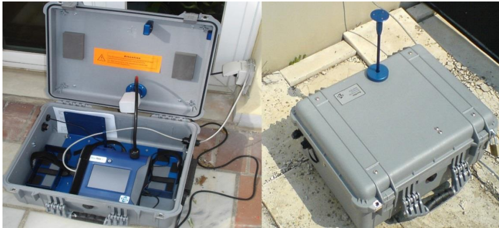
Figure 112 PM10 monitoring Instrument (Dustrak 8530) placed inside its environmental enclosure.
