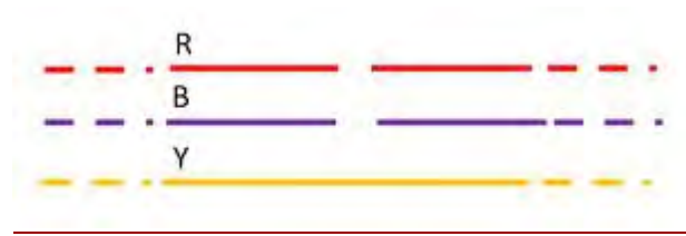
Figure 3.7 Two-phase open circuit [25]
