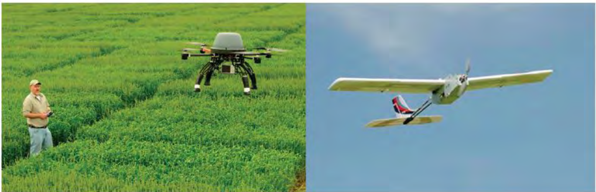
Figure 8. Two types of unmanned aerial vehicles: Rotary copter (left) and fixed-wing airplane (right).
