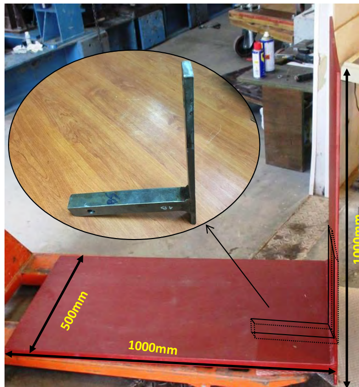
Figure 45. General view of a typical specimen, extracted from the large-scale welds.
